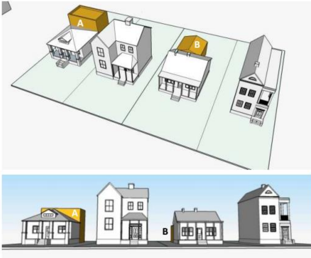
Adding a second story to a one-story dwelling is not appropriate as shown in example A. The rear addition in example B is a more appropriate solution for adding living space.
